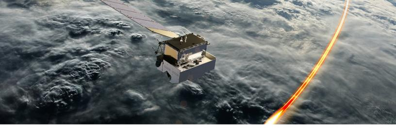
The Cross-track Infrared Sounder (CrIS) – an advanced spectrometer that produces high-resolution, three-dimensional temperature and moisture profiles from space – improves the accuracy of weather forecasting models for extreme weather three to seven days in advance, aids in "nowcasting" for thunderstorms and tornadoes, and improves understanding of longer-term weather and climate phenomena, such as El Niño and La Niña.
